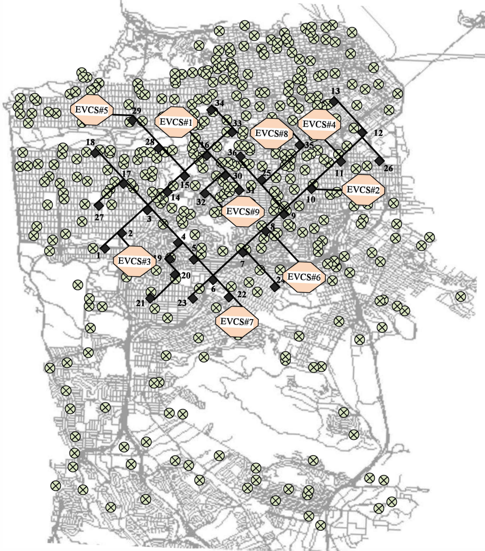
Figure 4: IEEE 37-bus distribution test network and location of some of the EVs and all CSs in San Francisco, the USA [49] and [50].
